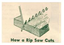
Appropriate cutting angle for rip and crosscut saws.
